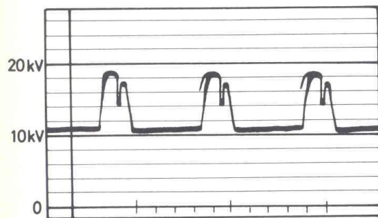
Break at one exciter diode.
