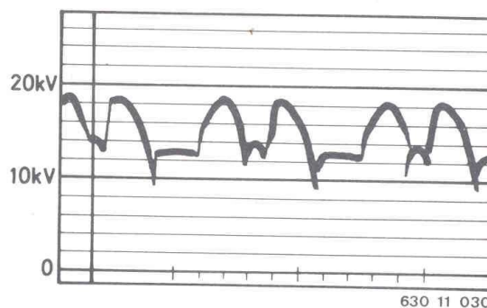
Short circuit at one positive diode.
