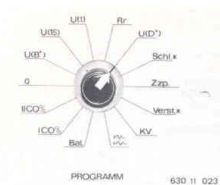
Switch position U (D+) 2000 \text{ min}^{-1} scale
